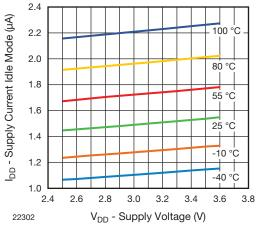
Fig. 2 - Idle Current vs. V<sub>DD</sub>
