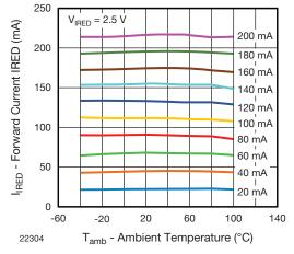
Fig. 4 - Forward Current vs. Temperature
