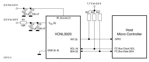
Fig. 9 - Application Circuit (x) = Pin Number
