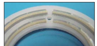
Circular Connector Grafted 160 Pos. (LCP Frame)
