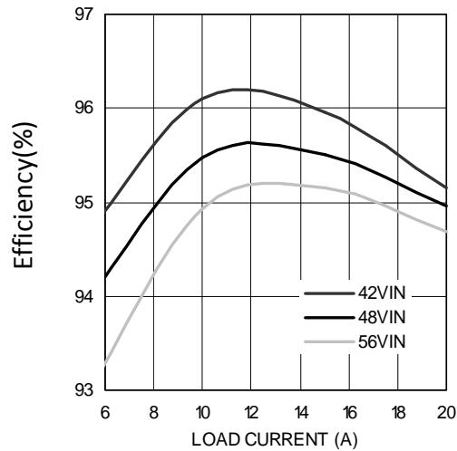
Figure 3. Efficiency with Pulse 1294.132 OR Inductor
