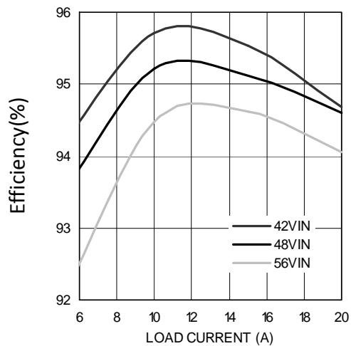
Figure 2. Efficiency with Demo Board Inductor
