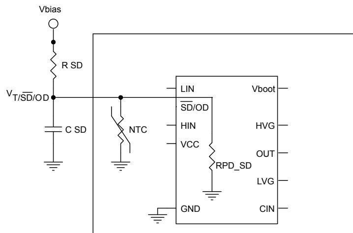
RPD\_SD: equivalent value as result of resistances of three drivers in parallel.
