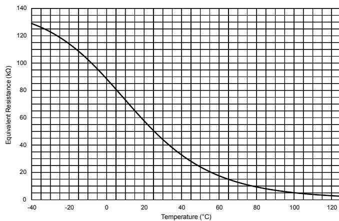
Figure 6. Equivalent resistance (NTC//R<sub>PD\_SD</sub>) zoom
