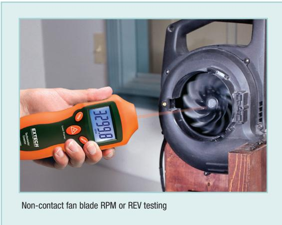
Non-contact fan blade RPM or REV testing
