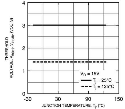
**THRESHOLD VOLTAGE VS. JUNCTION TEMPERATURE (TYPICAL - CONTROL PART P-SIDE)**
