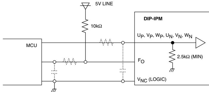
NOTE: RC coupling at each input (parts shown dotted) may change depending on the PWM control scheme used in the application and the wiring impedance of the printed circuit board. The DIP-IPM input signal section integrates a 2.5kΩ (min) pull-down resistor. Therefore, when using an external filtering resistor, care must be taken to satisfy the turn-on threshold voltage requirement.
