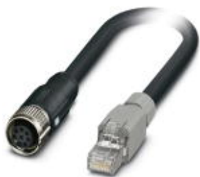
Bus system cable, VARAN, 6-pos., black halogen-free TPE, shielded, straight M12 SPEEDCON plug to RJ45 plug-in plug (IP20), cable length: 6 m
