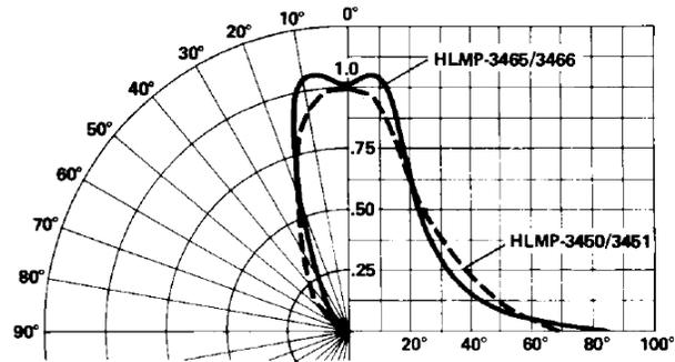
Figure 16. Relative luminous intensity vs. angular displacement.
