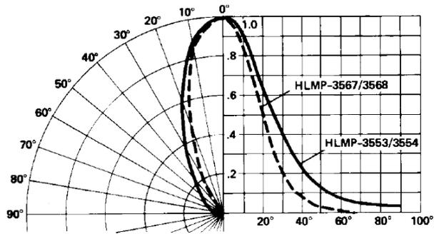
Figure 21. Relative luminous intensity vs. angular displacement.
