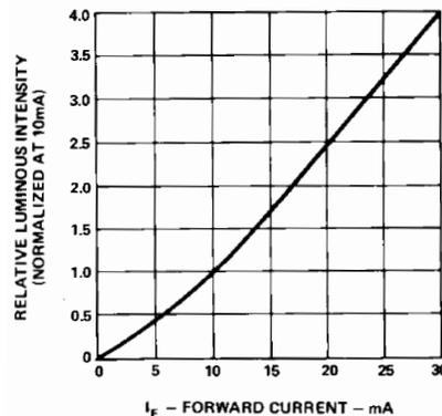
Figure 8. Relative luminous intensity vs. forward current.
