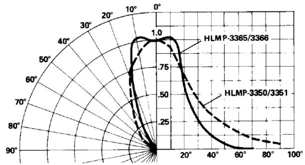
Figure 11. Relative luminous intensity vs. angular displacement.
