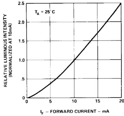
Figure 13. Relative luminous intensity vs. forward current.
