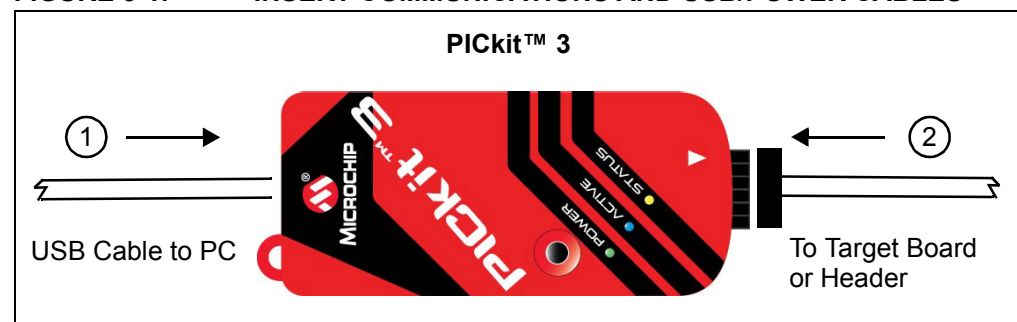
FIGURE 3-1: INSERT COMMUNICATIONS AND USB/POWER CABLES
