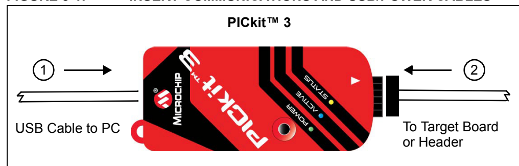
FIGURE 3-1: INSERT COMMUNICATIONS AND USB/POWER CABLES
