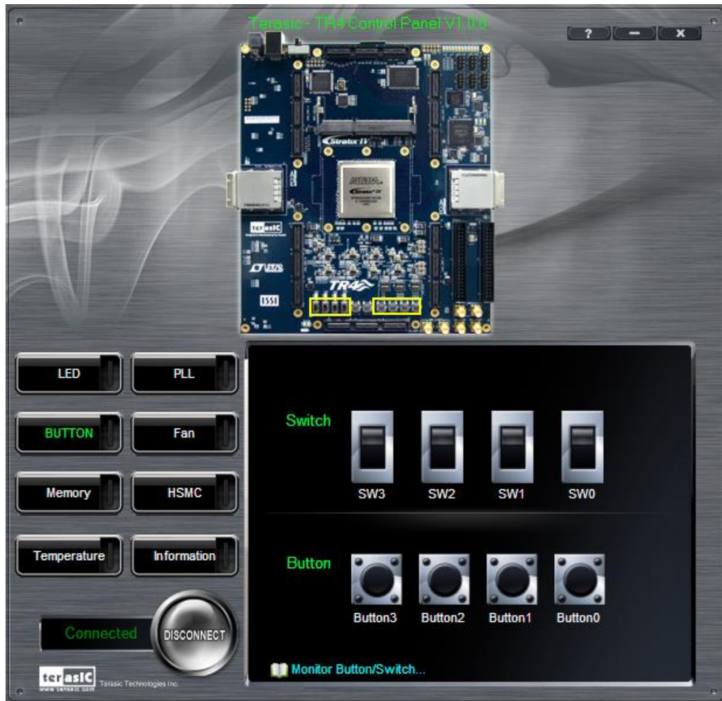
Figure 3-6 Monitoring Switches and Buttons
