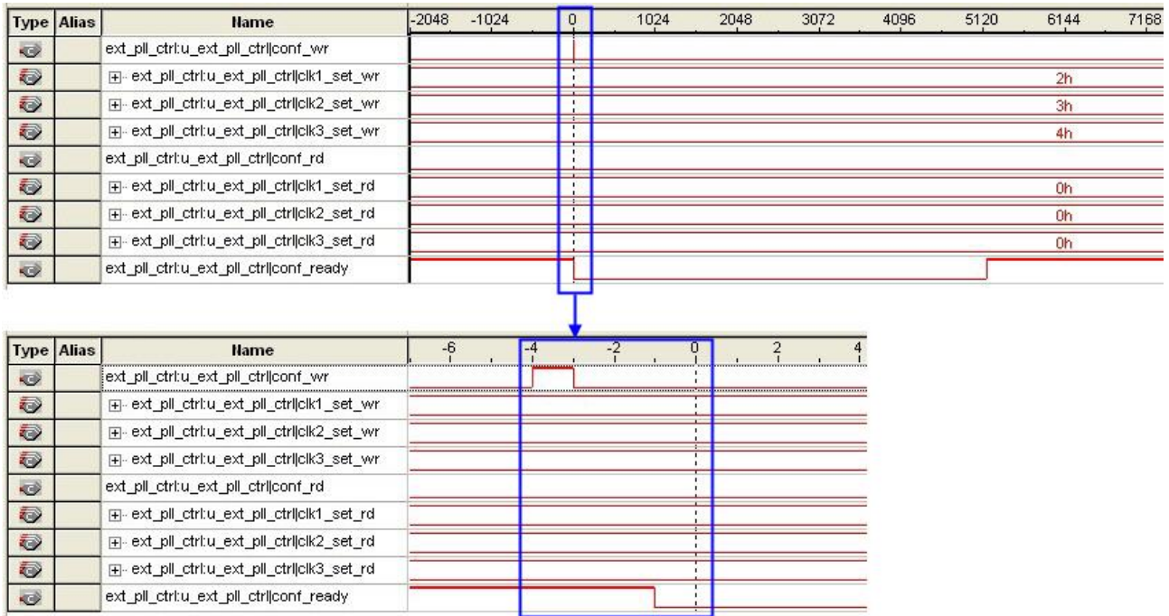
Figure 5-3 Write Timing Waveform
