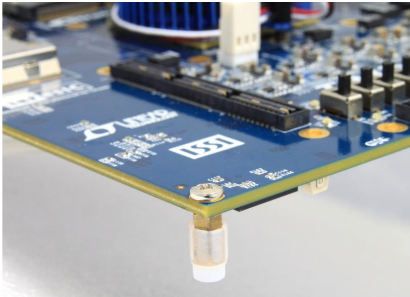
Figure 1-4 Mount Silicon Foot Stands
