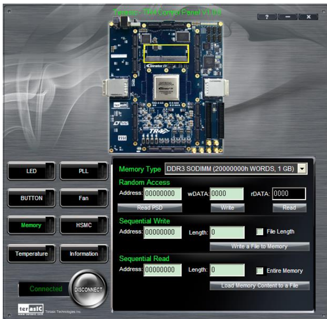
Figure 3-7 Access DDR3 SO-DIMM Memory
