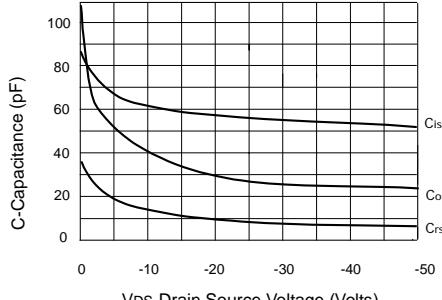
**Capacitance v drain-source voltage**
