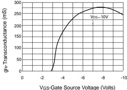
**Transconductance v gate-source voltage**
