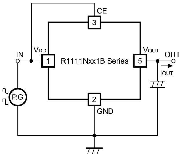
Fig.3 Ripple Rejection, Line Transient Response Test Circuit
