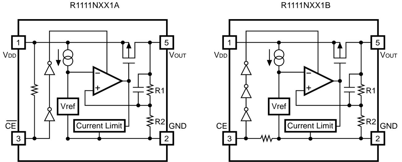
In these ICs, fluctuation of Output Voltage,  $V_{OUT}$  is detected by Feed-back Registers R1, R2, and the result is compared with a reference voltage by Error Amplifier, so that a constant voltage is output. A current limit circuit for Protection at short mode and a chip enable circuit are included.
