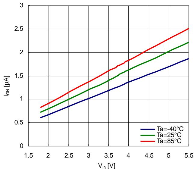
6) ON pin Pull-Down Current vs. Temperature
