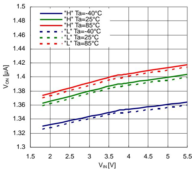
8) ON pin Logic Threshold vs. Input Voltage
