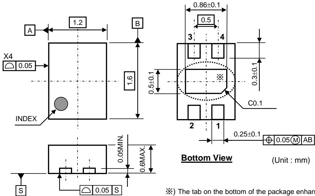
※) The tab on the bottom of the package enhances thermal performance and is electrically connected to GND (substrate level). It is recommended that the tab be connected to the ground plane on the board, or otherwise be left floating.
