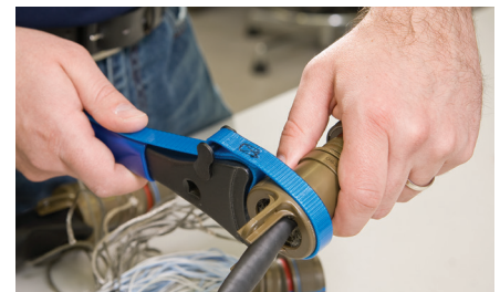
Strap wrench, strain relief, connector
