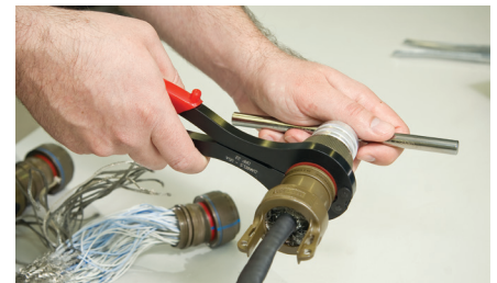
Circular Ring Pliers, strain relief, connector, adaptor, T-handle
