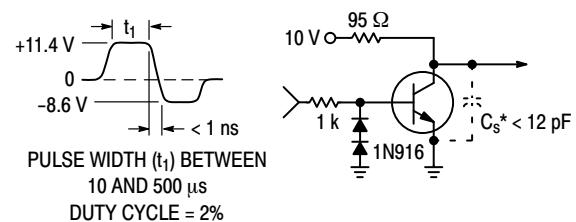
\*Total shunt capacitance of test jig and connectors.
