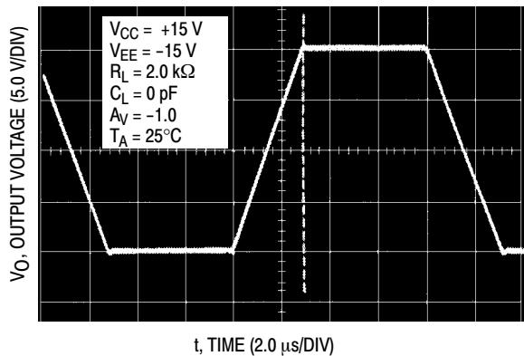
**Figure 21. Inverting Amplifier**
