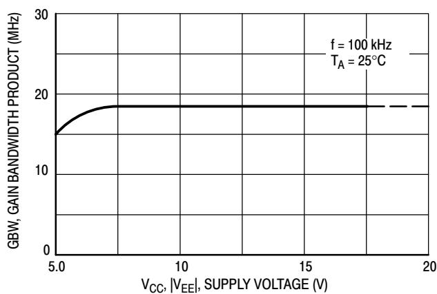
**Figure 9. Gain Bandwidth Product versus Supply Voltage**
