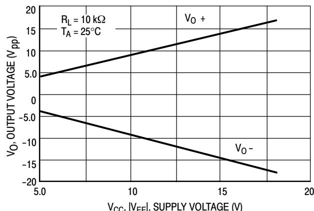
**Figure 13. Maximum Output Voltage versus Supply Voltage**
