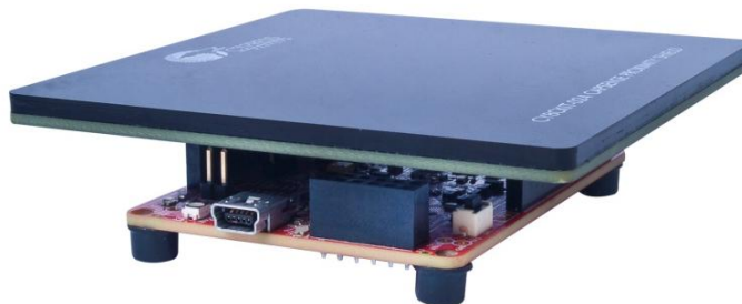
Figure 1-3: CY8CKIT-024 Connected to CY8CKIT-042
