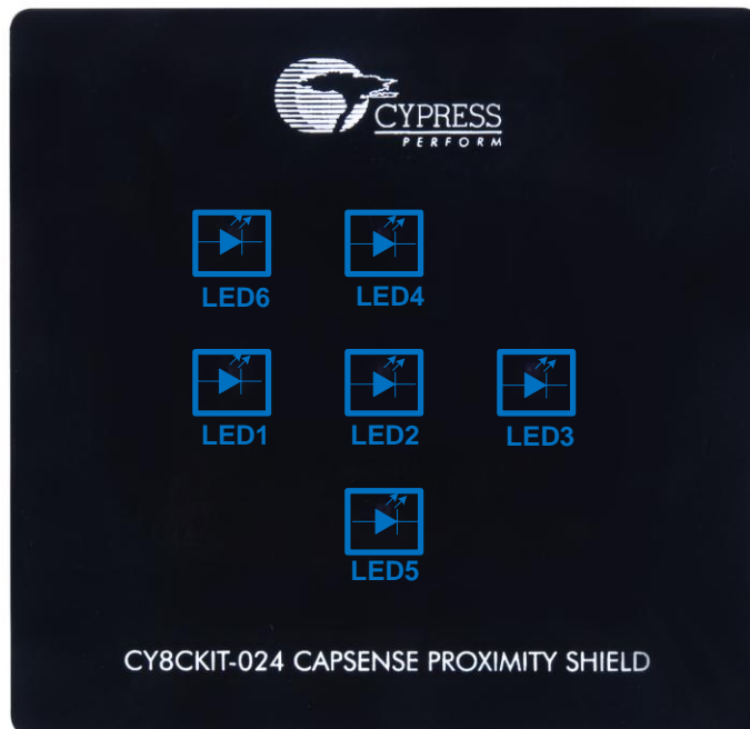
Figure 2-14: LEDs on CY8CKIT-024
