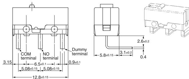
**● PCB Terminals (Left-angled)**
