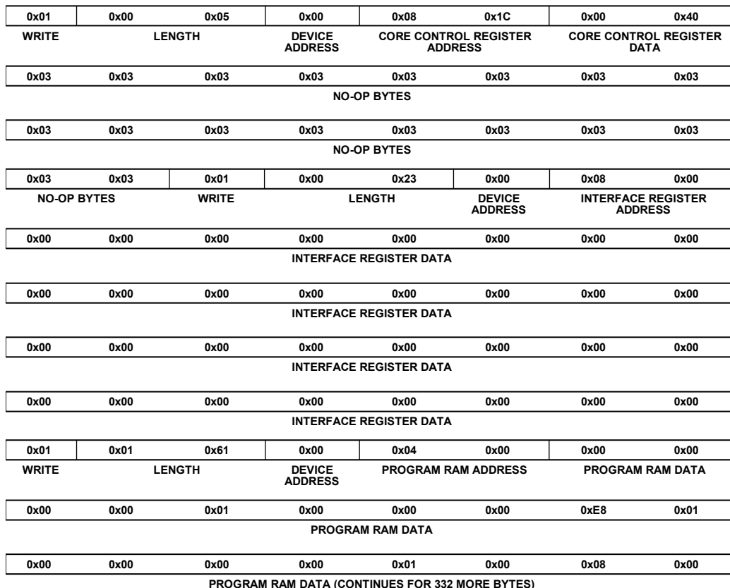
Figure 28. EEPROM Data Example
