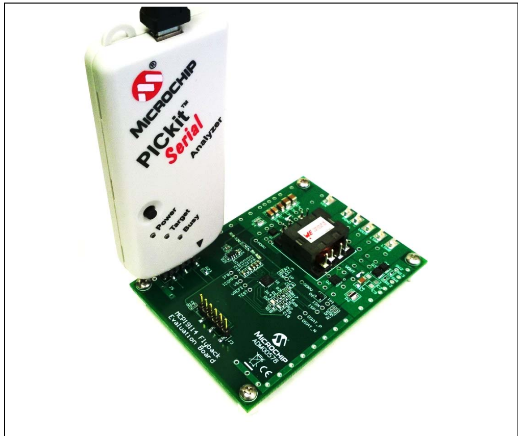
FIGURE 3-1: PICKit Serial Analyzer Connection to the Board.
