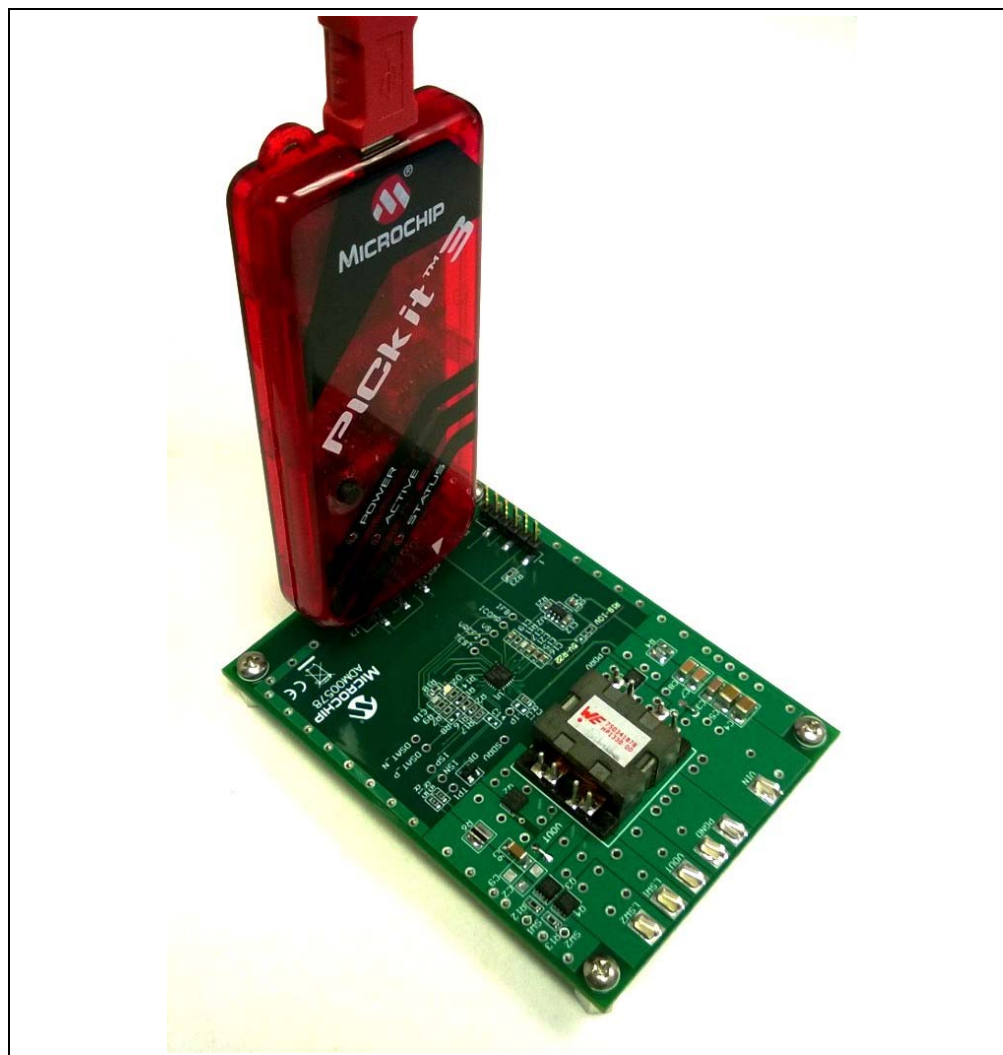
FIGURE 2-3: PICkit 3 In-Circuit Debugger/Programmer Connected to the MCP19114 - Flyback Stand-Alone Evaluation Board.
