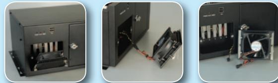
Step 1: Loosen the thumb screws
