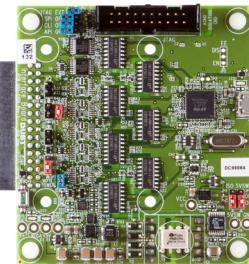
When connected to a DC9003A-B Evaluation/Development Mote, the **DC9006 Eterna interface card** provides a USB connection for both power and software access to the mote API UART port. The DC9006 comes with a DC9004 adapter card (not pictured) enabling the DC9006 to connect to the 10-pin programming and CLI header recommended for customer designs. Please see [www.linear.com/solutions/3102](http://www.linear.com/solutions/3102) for more details.
