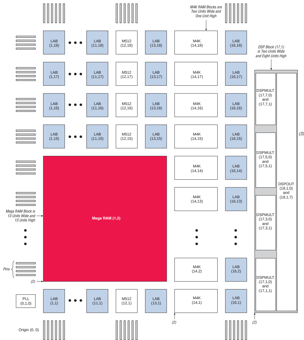
Figure 3–2. Stratix & Stratix GX Architectural Elements Note (1)
