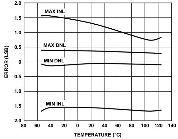
Figure 7. INL and DNL Error vs. Temperature
