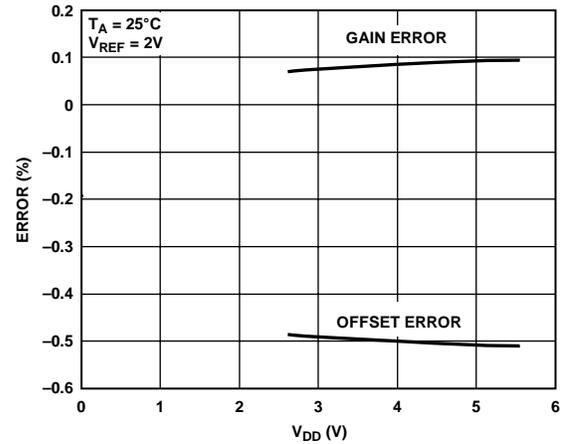
Figure 8. Offset Error and Gain Error vs.  $V_{DD}$
