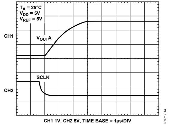
Figure 14. Half-Scale Settling (1/4 to 3/4 Scale Code Change)
