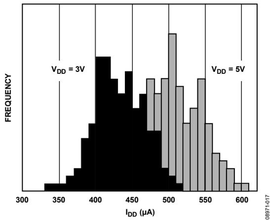
Figure 17. I<sub>DD</sub> Histogram with V<sub>DD</sub> = 3V and V<sub>DD</sub> = 5V
