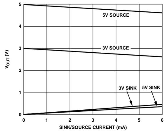
Figure 9.  $V_{OUT}$  Source and Sink Current Capability
