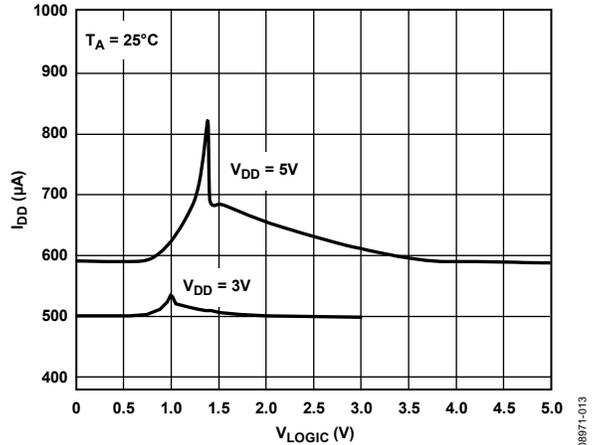
Figure 13. Supply Current vs. Logic Input Voltage
