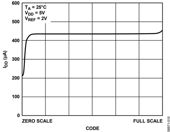
Figure 10. Supply Current vs. DAC Code
