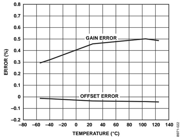
Figure 6. Offset Error and Gain Error vs. Temperature
