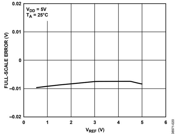
Figure 20. Full-Scale Error vs. V<sub>REF</sub>
