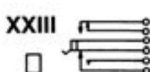
Single closed circuit plus "make" before "break". Isolated switching - "make" before "break" circuit. (J8-1D).
