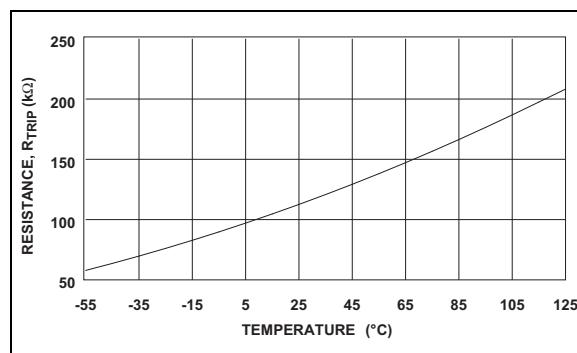
**FIGURE 3-2:** TC620 Sense Resistors vs. Trip Temperature
