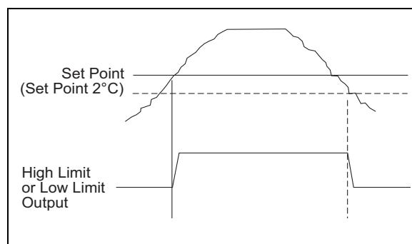
**FIGURE 3-3:** Built-In Hysteresis on Low Limit and High Limit Outputs
