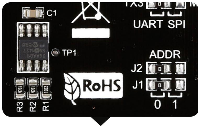
**Note** The BeagleBone click™ shield has an EEPROM module for storing pin configuration data. Initially the shield is configured with a blank EEPROM. The default address for the EEPROM is 0x54. You can change it to addresses 0x50 - 0x57 with the selection of the two address jumpers. They are Labeled A0 and A1. To write to EEPROM, use the onboard TP1 pin [which needs to be connected to GND].
