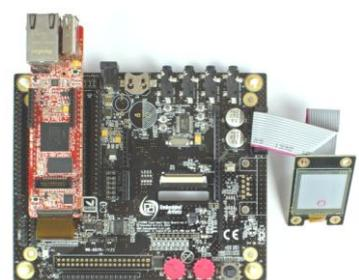
Figure 13 – LPC4088 Experiment Bundle, Displays and Serial Expansion Connector
