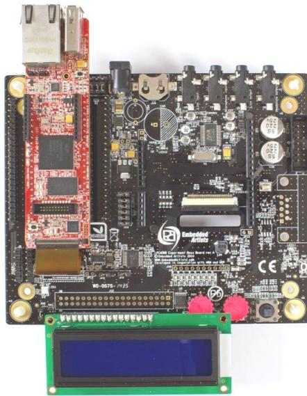
Figure 17 – LPC4088 Experiment Base Board, Character LCD
