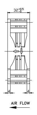
LEAD WIRES : UL 1007, AWG24 , L = 300 + -10 mmRed = positive ; Black = negative.
