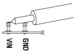
Figure 2. Measuring Input or Output Ripple
