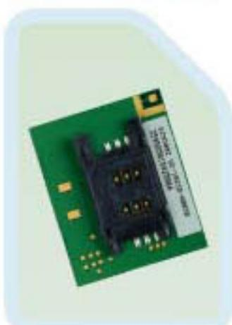
The SIM300E/340E is a Tri-Band/Quad-Band GSM/GPRS solution in a compact plug-in module.
