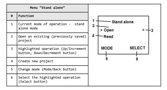
The options in this menu let you either open the program file located on the SD card or read the memory of the currently connected MCU.
