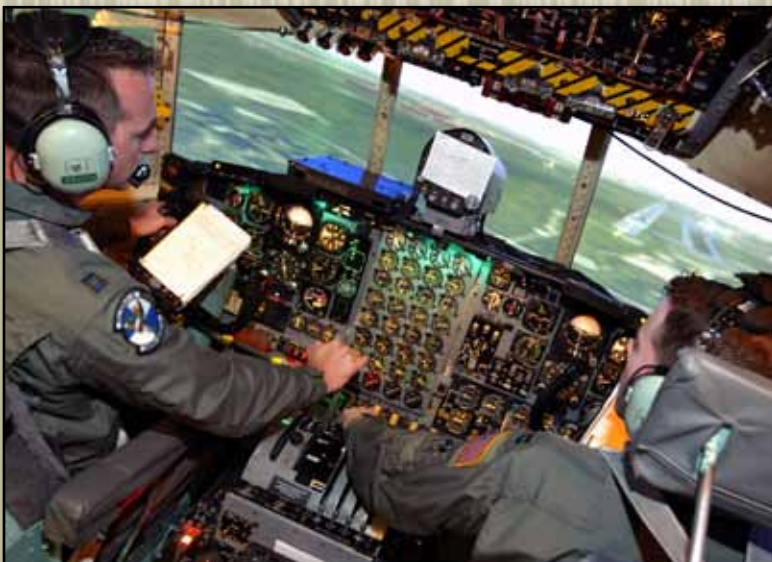
Cockpit avionics are susceptible to multiple sources of EMI including man-made interference from iPhones and other PEDs
