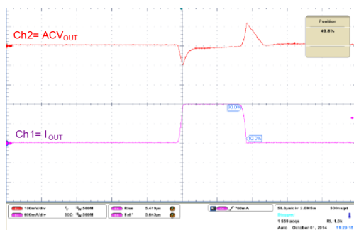
Figure 38. Load transient ( V_{OUT} = 5\text{ V} )
