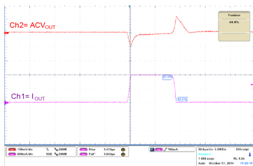
Figure 38. Load transient ( V_{OUT} = 5\text{ V} )
