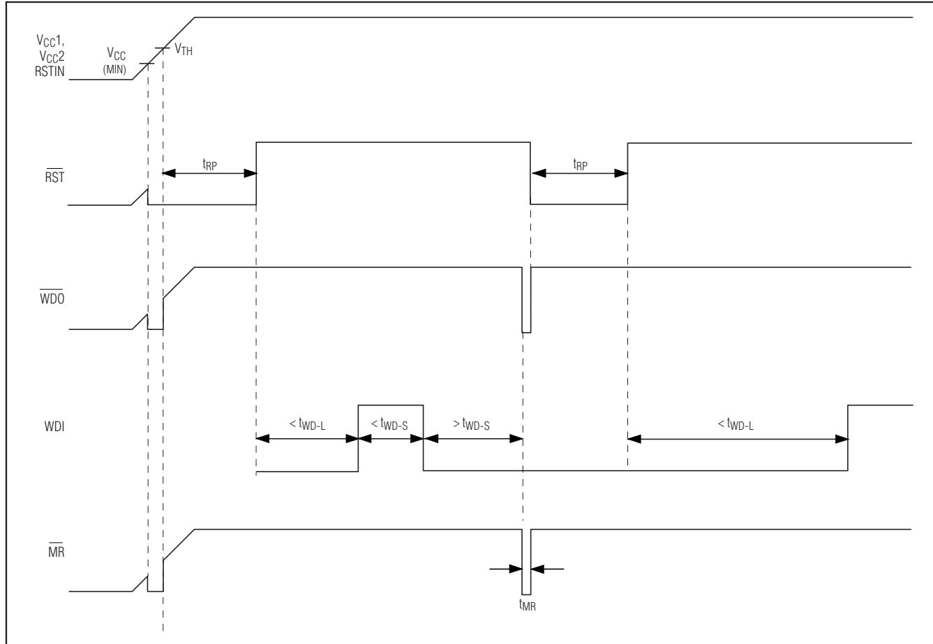
Figure 4. Watchdog Input/Output Timing Diagram ( $\overline{MR}$  and  $\overline{WD}\overline{O}$  Connected)
