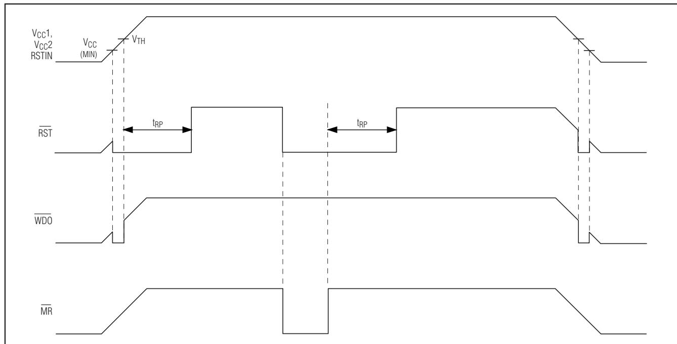
Figure 1. RST, WDO, and MR Timing Diagram
