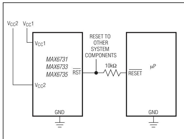
Figure 5. Interfacing to µPs with Bidirectional Reset I/O
