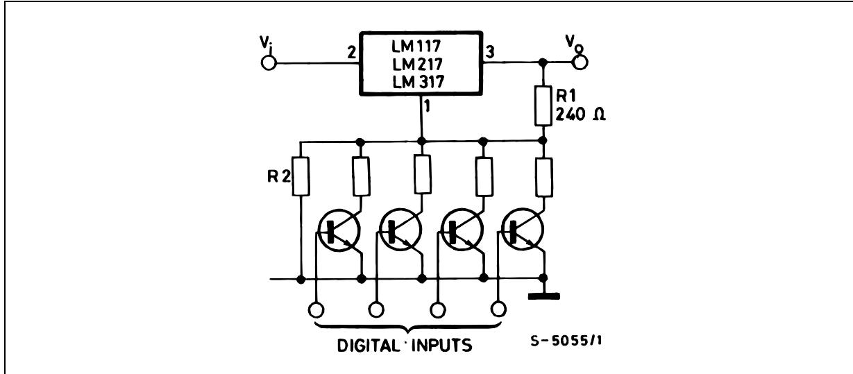
(R<sub>2</sub> sets maximum V<sub>O</sub>)**Figure 12.** Battery charger (12 V)
