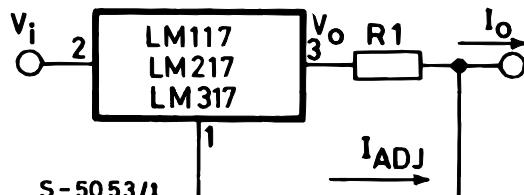
$$I_o = (V_{REF} / R_1) + I_{ADJ} = 1.25 V / R_1$$
