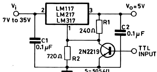
**Figure 11.** Digitally selected outputs
