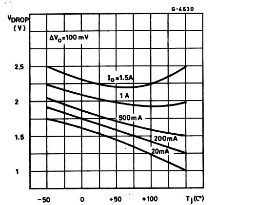
**Figure 5.** Reference voltage vs. junction
