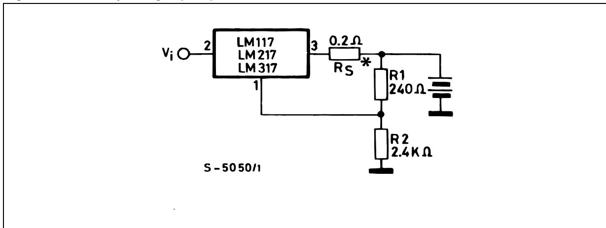
\*  $R_S$  sets output impedance of charger  $Z_O = R_S (1 + R_2/R_1)$ . Use of  $R_S$  allows low charging rates with fully charged battery.
