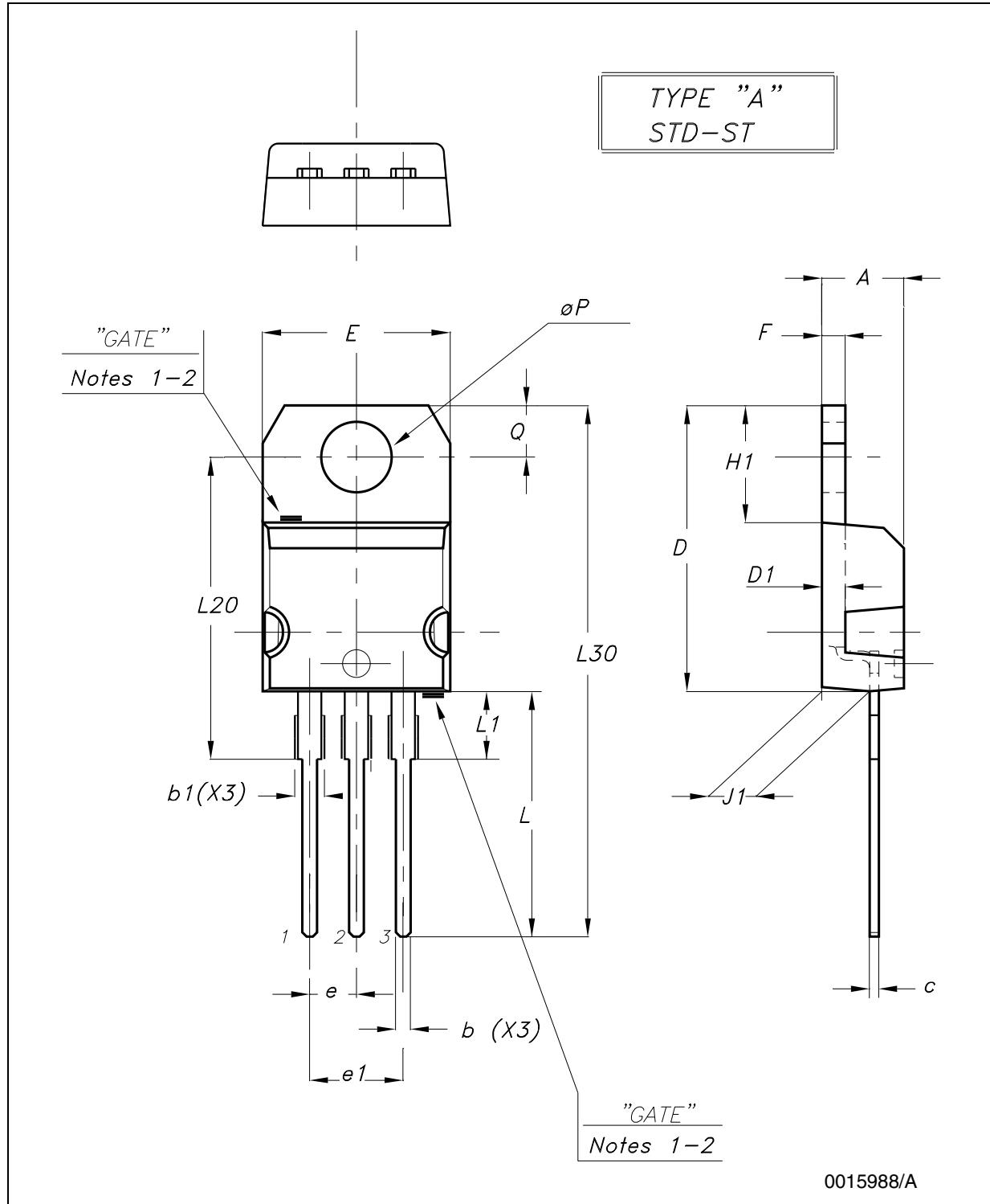
Note: 1 Max resin gate protrusion: 0.5 mm.
