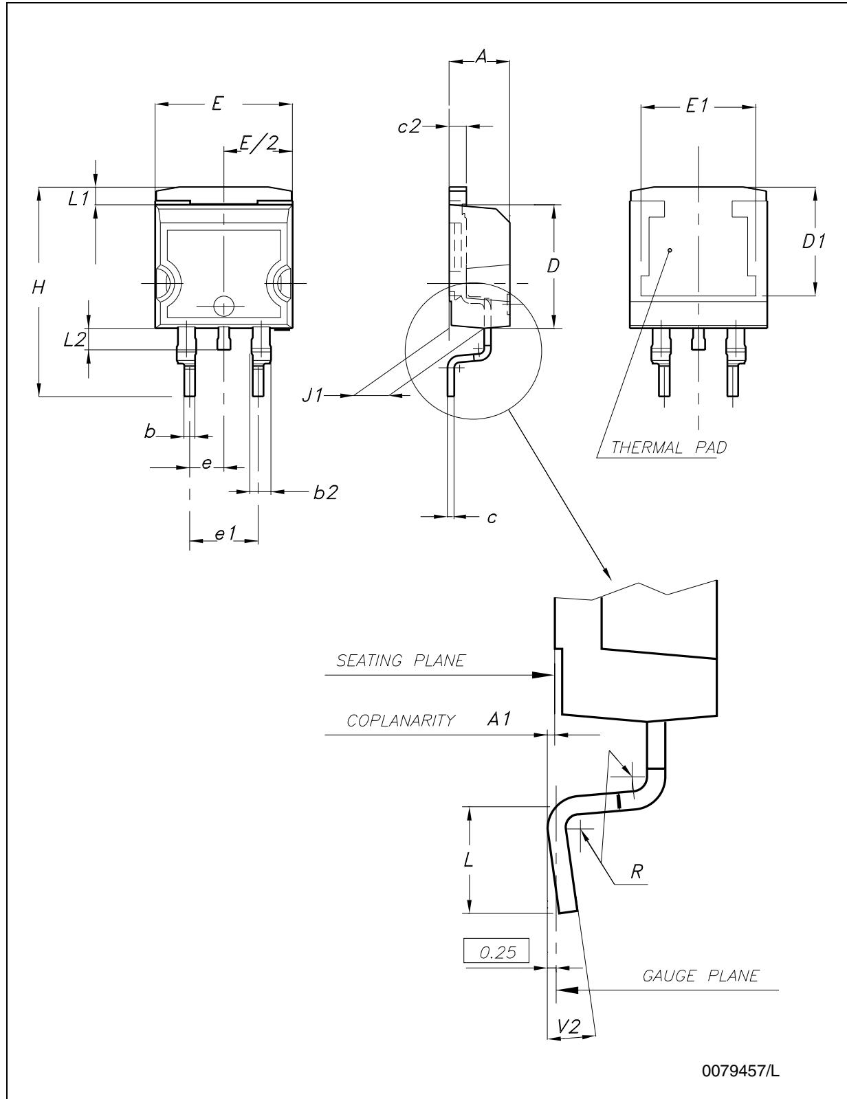
**Figure 19.** Drawing dimension D<sup>2</sup>PAK (type WOOSEOK-SUBCON.)
