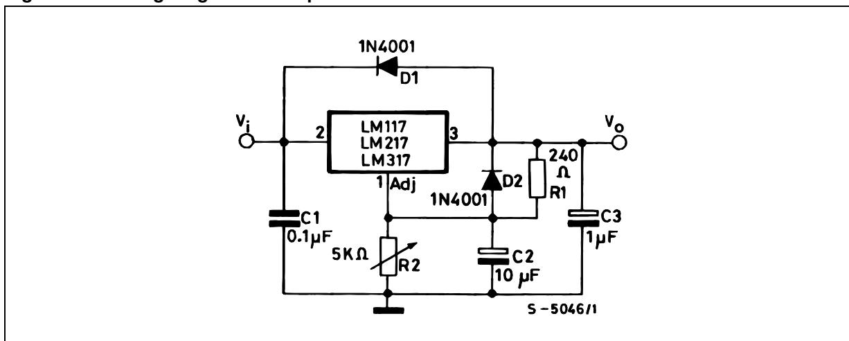
Note: D1 protect the device against input short circuit, while D2 protects against output short circuit for capacitors discharging.
