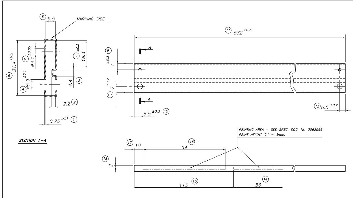
**Figure 17. Drawing dimension tube for TO-220 Single Gauge (mm.)**
