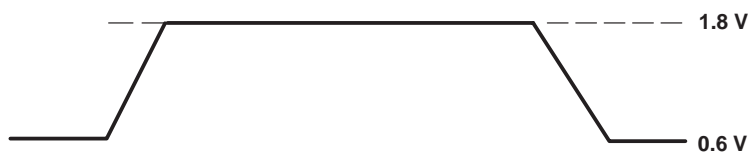
Figure 9. 'LC31 Input Levels
