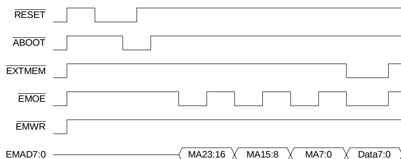
Figure 35. Autoboot Timing Diagram
