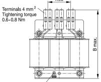
PE M4 / Tightening torque 1.2±0.1 Nm
