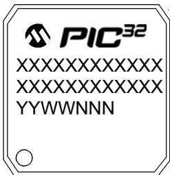
100-Lead TQFP (12x12x1 mm)
