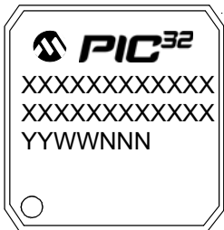
100-Lead TQFP (12x12x1 mm)
