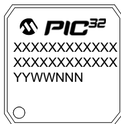
100-Lead TQFP (14x14x1 mm)
