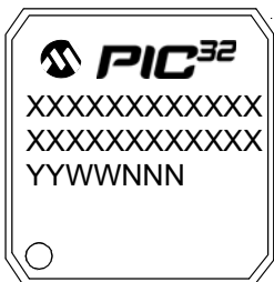
100-Lead TQFP (12x12x1 mm)
