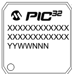
100-Lead TQFP (14x14x1 mm)
