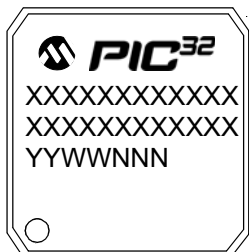
100-Lead TQFP (12x12x1 mm)
