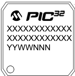
100-Lead TQFP (12x12x1 mm)
