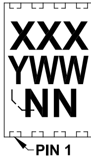
8-Lead TDFN (2x3x0.75 mm)
