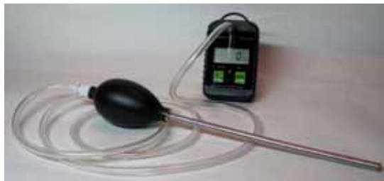
Accessory probe with squeeze-bulb sample pump offers effective flue gas combustion analysis as well as troubleshooting of burners, heat exchangers, and exhaust ducts
