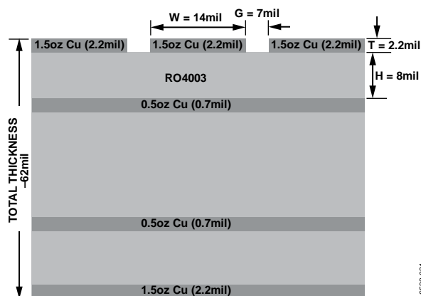
Figure 22. Probe Matrix Board (Cross Section View)
